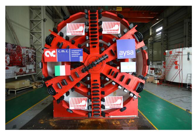
The tunnel will be excavated at an average depth of 25m, beginning with an approximately 400m radius curve and continuing along an essentially straight alignment, reaching a maximum slope of +/- 2.0%. As the machines progress, they will install a precast concrete segmental lining ring consisting of six (four parallelograms and two keys) 250mm thick, 1400mm wide, segments.
